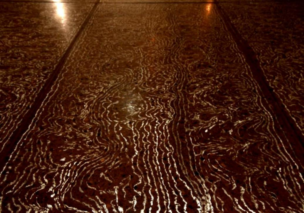
The patent protected Litracon® products present the phenomenon of light transmitting concrete in form of widely applicable new building materials. They have been being developed by Hungarian architect Áron Losonczi since 2001.
